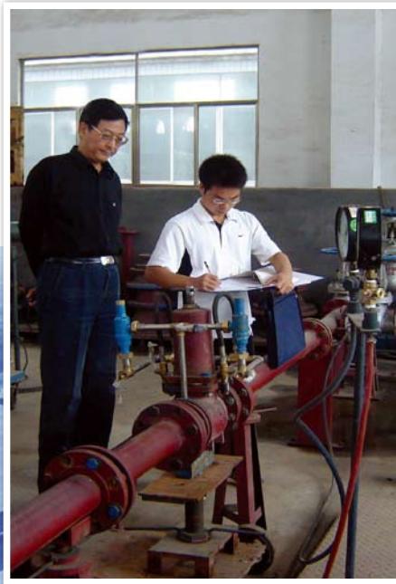
湖南省技术监督局的工作人员在做流量特性实验 Experiment on flow characteristics by staff from Bureau of Technical Supervision of Hunan Province
